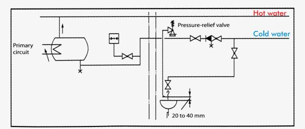
Installation of complete safety system and water heater in different rooms
