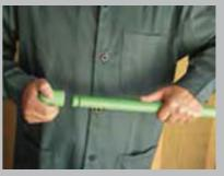
Timing for heating should not start until the pipe and fitting reaches to the marked welding depth. Both fitting and pipe should be heated for a set time, known as the heating time.
